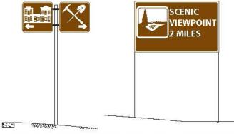
(z) Directional signs an State or Caunty roads use a family (z) Signs far a af ixanic symbols along with a directional arraw. This type of two symbol af sign uses a maximum of faur symbols.
